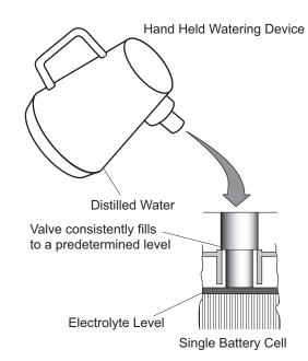
NOTICE: The watering device should only be used if the electrolyte level is less than 1/2" (13 mm) above top of plates.
