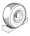
With the valve stem to the outside, mount the wheel onto the hub with the lug nuts. Finger tighten the lug nuts (1) in a 'cross sequence' pattern. Tighten the lug nuts to 65 to 75 ft. lbs. (88 to 101 Nm) torque in 20 ft. lbs. (27 Nm) increments following the 'cross sequence' pattern.
