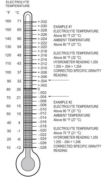
Hydrometer Temperature Correction
