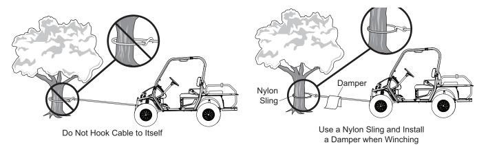
Stay clear of the winch, cable and cable hook. Place a heavy cloth, jacket or blanket over the cable to act as a damper should the cable break when operating the winch.
